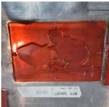
NEW CYREL USING HARD CYREL ON THE CRITICAL CHARACTER PRINT
