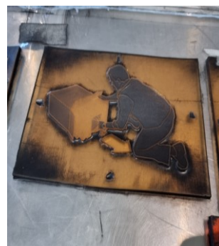
OLD CYREL USING SOFT CYREL ON THE CRITICAL CHARACTER PRINT
