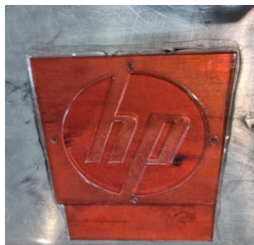
NEW CYREL USING HARD CYREL ON THE CRITICAL CHARACTER PRINT
